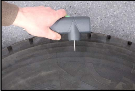
Best orientation for picking up RFID tags in a tyre sidewall.
